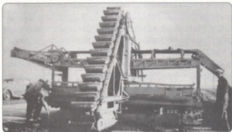
Figure 8: The earliest known machine to use stringline technology was the A. W. French Utility Grader. A. W. French & Company sales literature
